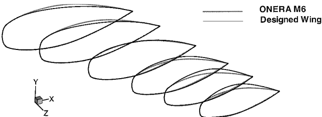
Fig. 5 Geometries of the ONERA M6 and designed wing.
